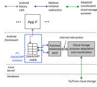
Fig. 4. App runtime instrumentation based implementation overview.
