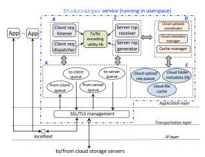
Fig. 3. Implementation of the user-level StoArranger service.
